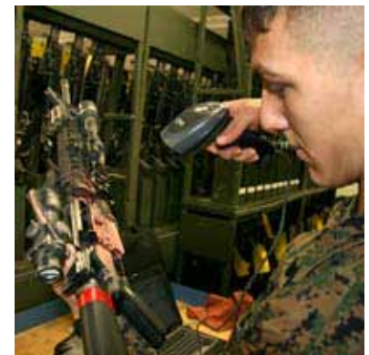
Corporal Bryan McLain scans the weapon's IUID label at The Basic School Armory on Marine Corps Base Quantico, Va.
